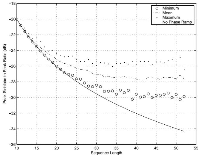
Fig. 4. Side-lobe levels of polyphase Barker codes after injecting 0.25 deg. of phase per chip
