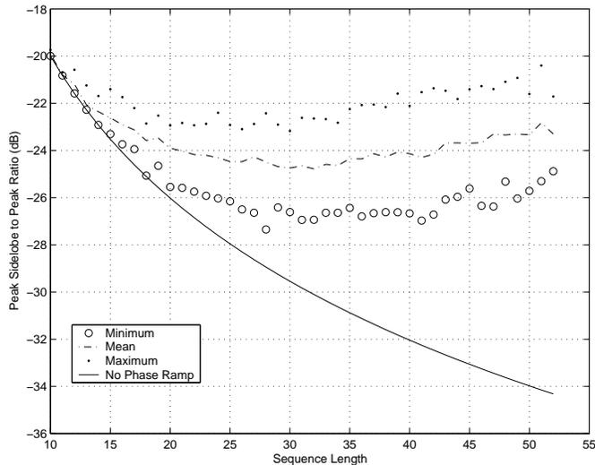
Fig. 5. Side-lobe levels of polyphase Barker codes after injecting 0.50 deg. of phase per chip
