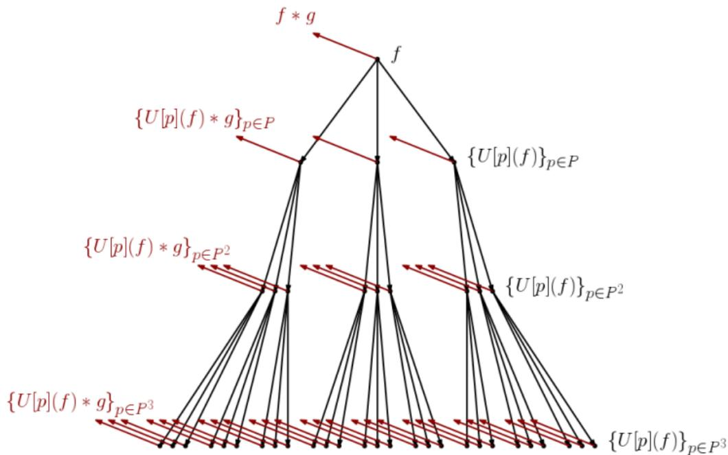
Figure : Network structure of the scattering transform.
