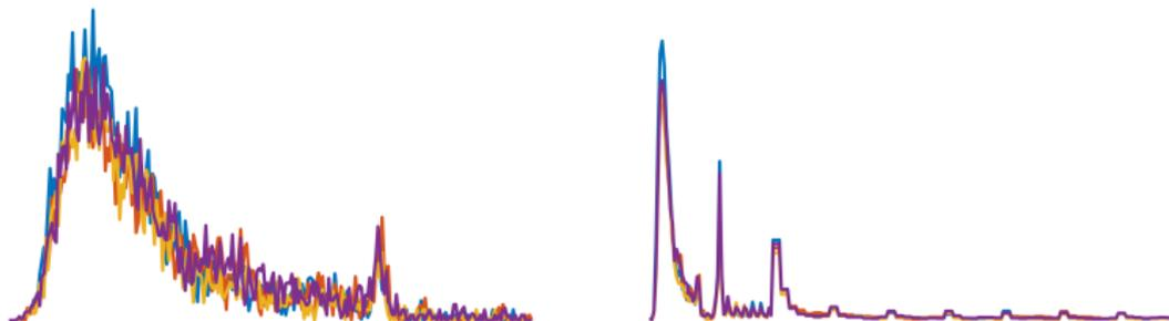
**Figure** : Raw gamma spectrum (left) and their corresponding Fourier scattering spectra (right). The red, blue, and yellow gamma spectrum were taken near each of the three sources, while the purple spectra was taken far away.
