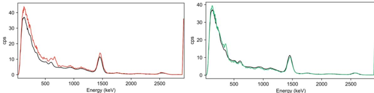
Figure : Gamma spectrum for cs (left) and pus (right).
