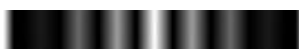
Figure 3.2: A diffraction pattern created by the constructive and destructive interference of light from two point sources.
